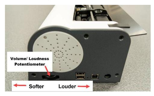
Note that the volume dial can also be used to move the paper up or down one braille dot at a time if used while pressing the space bar.
