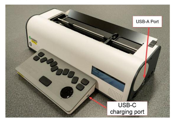
To check keyboard battery status, press the K Chord (Space and dots 1 and 3 at the same time).
