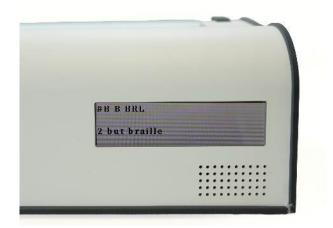
Some students may find the LCD screen distracting; however the screen cannot be turned off. If the screen is an issue, one option is to tape a piece of cardboard, or place a sticky note over the screen in a way that it will still be easily accessible when you need it.
