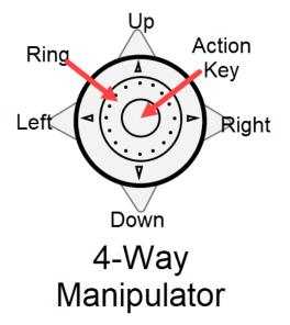
You can scroll through the menu items by pressing the up and down arrows, or by scrolling the Ring clockwise and counterclockwise.
