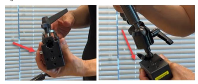
To attach to a flat surface, move the wedge from where it is stored and place it in the jaw of the Super Clamp. This will provide extra clamping surface.
